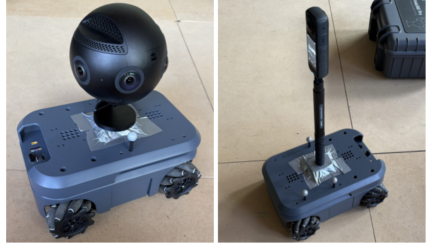
Figure S1. The Insta360 Pro mounted on the Elephant robotics myAGV robot (left). The mounted Insta360 X4 camera using a telescopic extension stick (right). A 1/4-20 UNC connection point was attached to the top side of the robot to mount the cameras.
